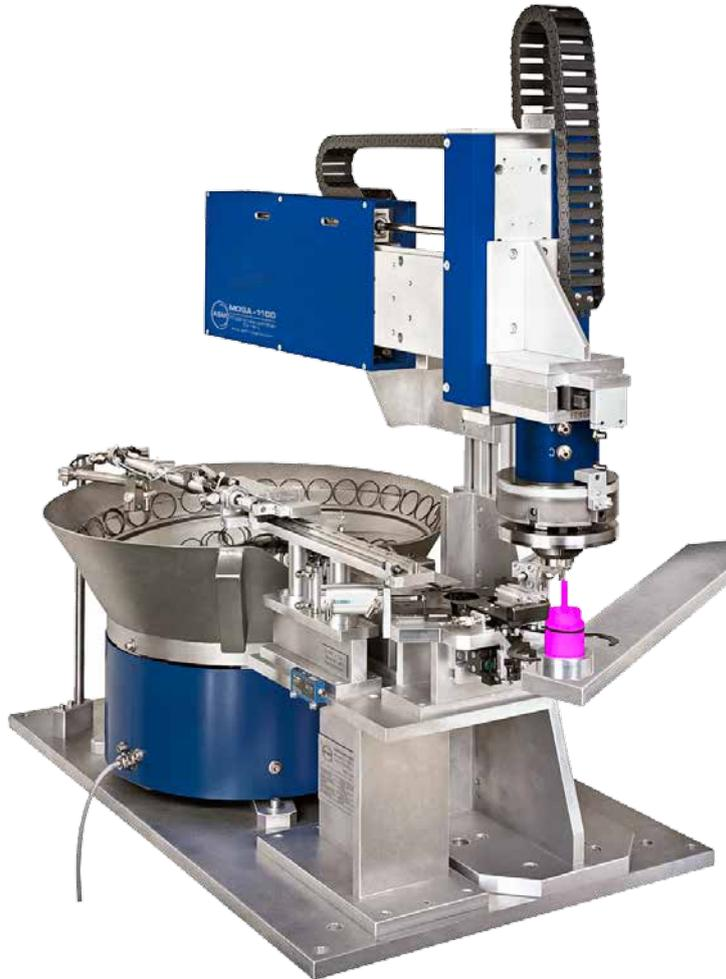
**Prep unit for the automatic provision and assembly of external sealing rings.**
